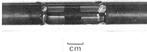
Fig. 4 Central enameled section of mild steel cylinder, with painted film and tags
