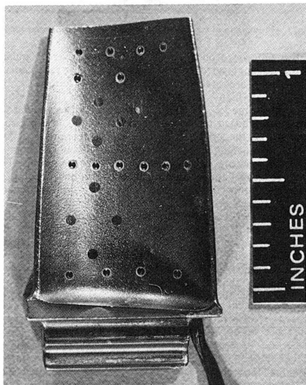
Fig. 3 Photograph of button-type gages on blade pressure surface
