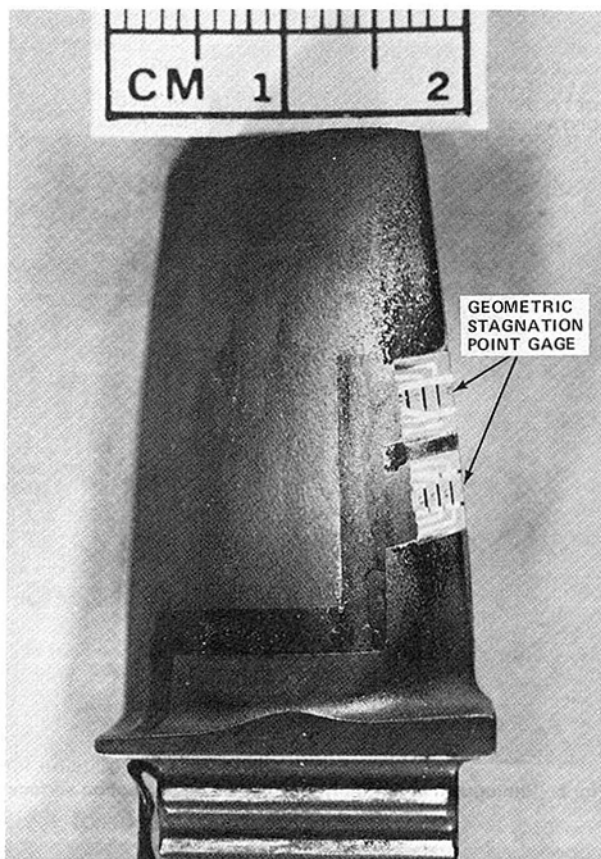
Fig. 1 Photograph of contoured leading-edge inserts for rotor blade
